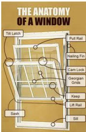
This window is called "double hung". Both the top & the bottom panes slide up & down. On a single hung window, only the bottom slides up & down. It looks like these muntins are in between the glass. That's called a "dual pane" window. It has 2 panes of glass, with an insulating gas in between. Dual pane windows are more energy efficient and reduce outside noise
